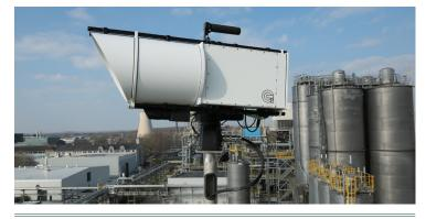
**Figure 2.** Grandperspective's sensors are able to continuously and autonomously identify, monitor and quantify hundreds of gases – including methane, ammonia and ethylene.
