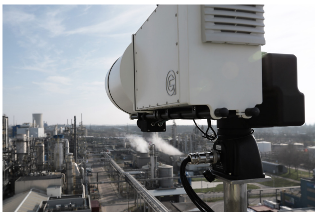
Figure 3. Mounted in an elevated position, the sensor unit continuously monitors large areas for dangerous emissions. One significant advantage of the system is that it operates completely independently of weather conditions.
